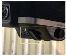
6. Remove the internal camera lens cover, secure any loose cables with cable ties and place tamper seal on all connections.
