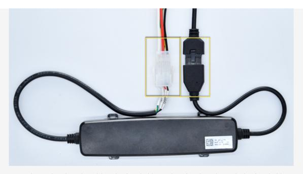
B. Insert the 2A fuse into the White wire fuse holder and 5A fuse into the Red wire fuse holder.
