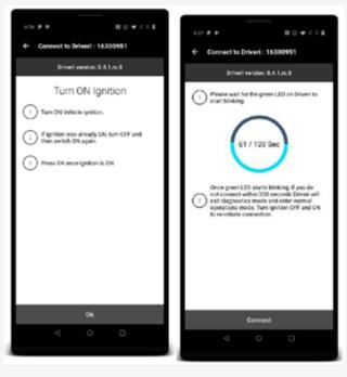
Enter the provided username, password, and device serial number. Once connected, click Camera and check both Road and Driver Cameras.
