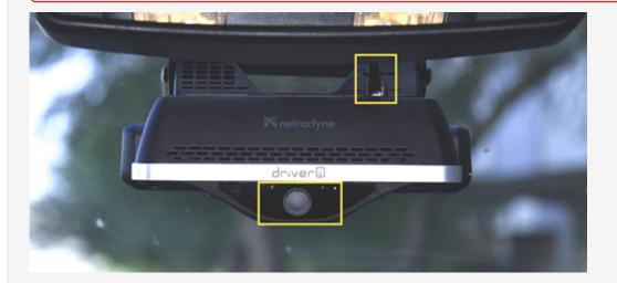
1. Place the device into the mounting bracket and lightly screw in the mounting bolts. Do not fully tighten down screws as the camera may need to be adjusted in Step 3.
