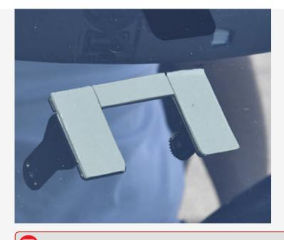
**Note.** Mounting brackets are one time use and should be thrown away after removal. Please contact your account manager for ordering additional mounting brackets.
