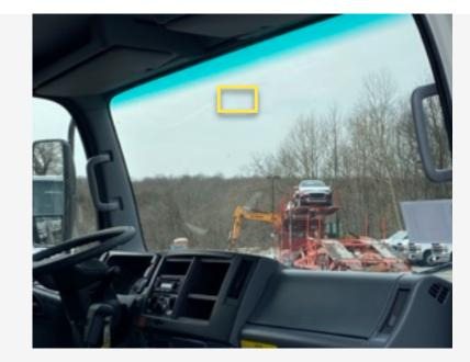
• Type 4: Angled/Split Windshield; Right windshield, down ~4-6" down from roof and ~1"in right of the center divider.
