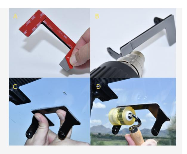
2. From outside the vehicle, visually inspect tape adhesion. There should be no air bubbles in the tape. If necessary, repeat the rolling process until required results are achieved.
