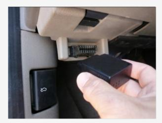
b. Secure the device to the OBD-II Port with a zip tie and ensure connection secure.
