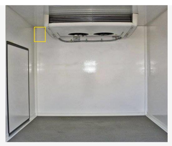
2. Identify a cable route from the temperature sensor location to the GPSI-3900. The cable placement should not prevent the use or removal of asset panels and should not leave the cable open to damage.
