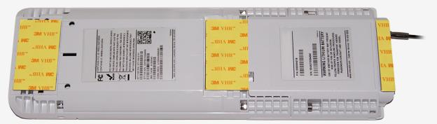
6. Using the supplied plastic nut wrench, remove the six nuts and remove the device from the studded brackets, and then apply firm pressure to each of the studded brackets for at least 60 seconds.
