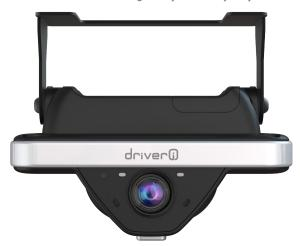
Driveri® is a smart camera, installed in trucks/cars behind the rear-view mirror. The power is supplied from the car battery through a custom power cable. The device is capable to connect with the OBD/J1939 of the vehicle to collect the vehicle data. This device is passive to the driver.
